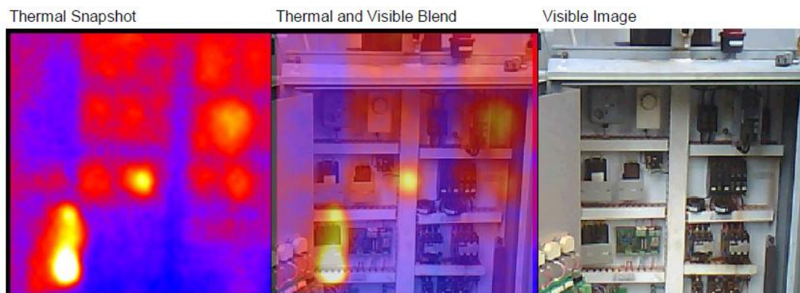
Control Panel Thermography Inspection Results
